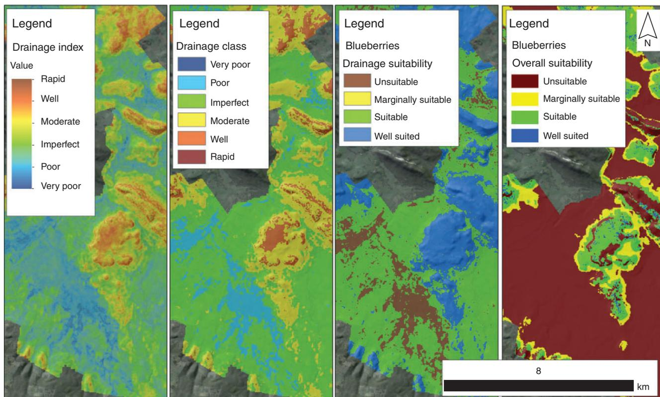
Fig. 4. Partial extent—Meander drainage index, classified drainage class, blueberries drainage suitability and blueberries overall suitability.
