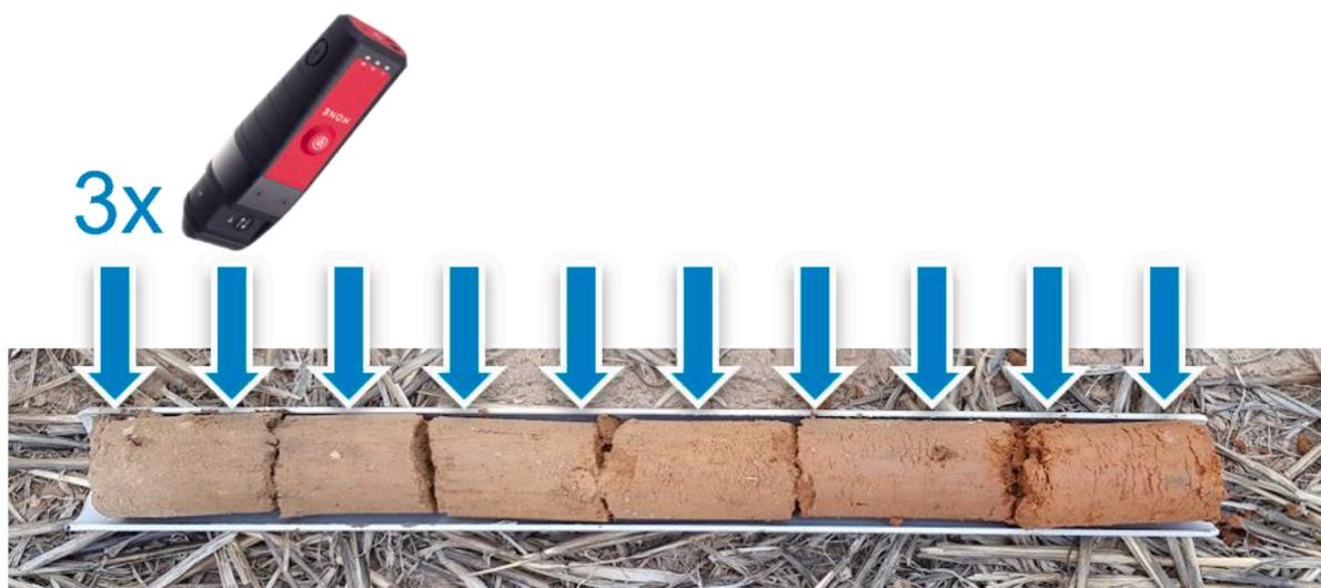
Fig. 3. A diagram displaying a field condition soil core, with 10 arrows distributed in 5 cm increments to demonstrate the collection of spectral information.
